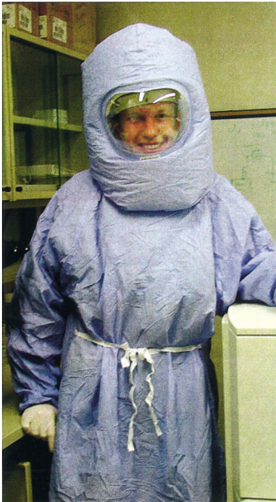
FIG. 4. The ProVison Personal Protection System. These photographs show the ProVison Personal Protection System and its mechanical helmet. The helmet consists of a battery-powered blower, which constantly moves room air through a 0.1- \mu\text{m} HEPA filter in the top of the suit. The respiratory suit as shown is a full-body suit with complete face protection and, when worn with gloves and boots, protects hands and feet from contamination during a viable infectious sort procedure.
